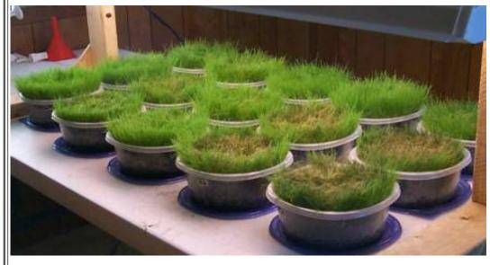
The front four test plots showing the burnt bentgrass are the result of petroleum hydraulic spills. The petroleum oils in these plots burned the grass within 24 hours. The remaining plots are spills of RLI's biobased hydraulic formulations, pure vegetable oil, and blank test controls. There was no noticeable difference in plant health between equal spill volumes of RLI's biobased hydraulic
